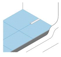
4. Commence with tiling using an appropriate ARDEX tile adhesive. Use a flat trowel to skim a coat of tile adhesive to the top mesh of ARDEX UD 150 ensuring that mesh is fully covered before troweling adhesive adhesive with a minimum notch size of 12mm.
