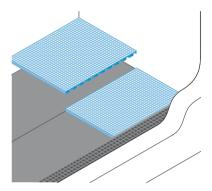
3. Install ARDEX UD 158 tape to join and reinforce all butted seams.
