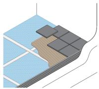
6. Install ARDEX Grout in accordance with the relevant datasheet.
